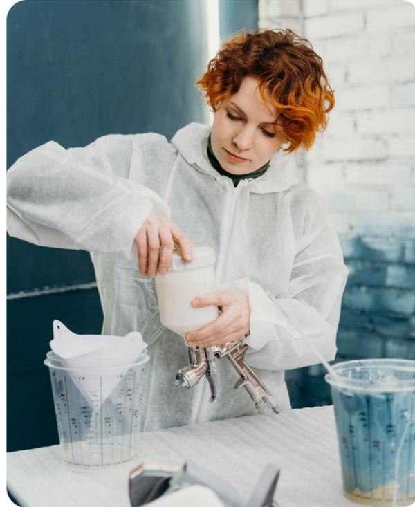
Mix your material components as you would normally and simply load in to the spray gun as required, this operation sometimes demands two operators as it's most sensible to mix smaller batches to eliminate materials hardening in the bucket prior to spraying.
