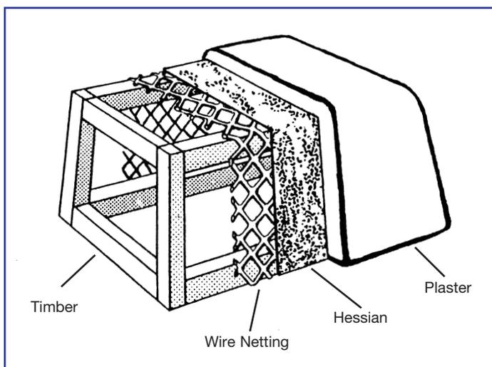
Typical construction of large plug – timber, wire netting, hessian and plaster.
